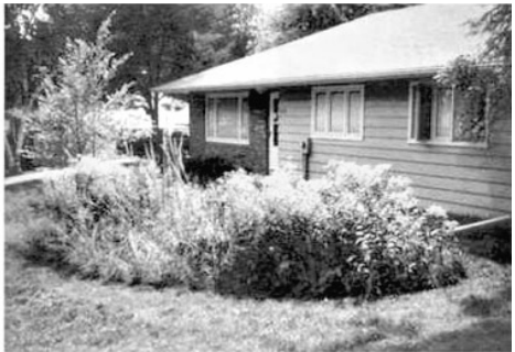
Rain gutters direct rooftop runoff to this attractive rain garden reducing stormwater problems for the homeowner and neighbors
